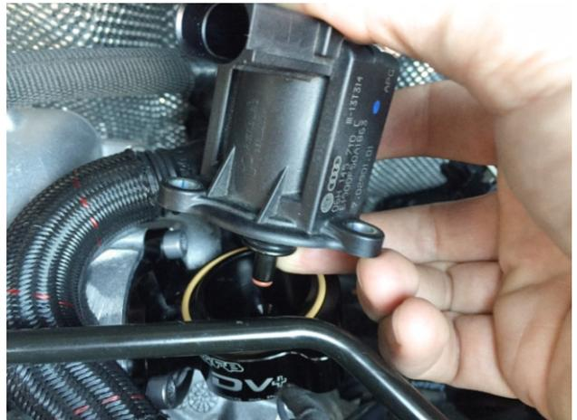
Fasten the solenoid using 3 screws (GFB or factory screws, they are the same). Re-install the turbo intake elbow, intake pipe, breather hose, and electrical connector in the reverse order of disassembly.
