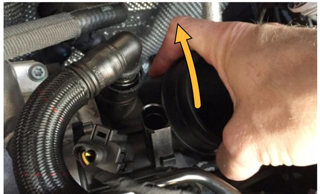
Now unscrew the 3 bolts holding the diverter valve (5mm metric hex key), then remove it from the car. Again, take care not to drop these screws as they can be difficult to retrieve. A driver extension with a 5mm hex bit can make it easier to remove and re-install these screws.
